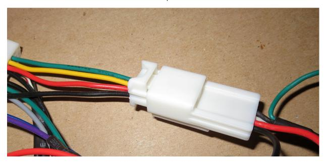
Other harnesses will be delivered with only the male connector. If your harness was delivered with the female connector, it will not be used for this application. Disconnect the 5-pin male and female connectors.
